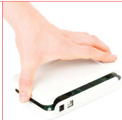
Figure 8-3: Place plastic casing cover and wind screws into outer screw holes to fix it with bottom plastics casing
