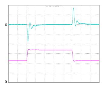
Figure 7: Output voltage response to step-change in load current (50%-75%-50% of lo, max; di/dt = 0.1A/µs; Vin is 48V). Load cap: 10µF tantalum capacitor and 1µF ceramic capacitor. Top Trace: Vout (0.2V/div, 200us/div), Bottom Trace: lout (2A/div). Scope measurement should be made using a BNC cable (length shorter than 20 inches). Position the load between 51 mm to 76 mm (2 inches to 3 inches) from the module
