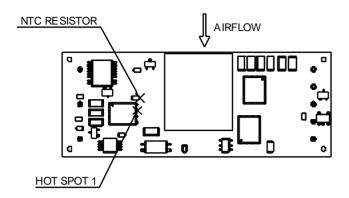
**Figure 19:** \* Hot spot 1& NTC resistor temperature measured points. The allowed maximum hot spot 1 temperature is defined at 115  $^{\circ}$
