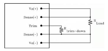
Figure 16: Circuit configuration for trim-down (decrease output voltage)
