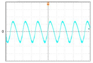
Figure 12: Output voltage ripple at nominal input voltage (Vin=48V) and rated load current (Io=9A) (20mV/div, 2us/div).Load capacitance: 1μF ceramic capacitor and 10μF tantalum capacitor. Bandwidth: 20 MHz. Scope measurements should be made using a BNC cable (length shorter than 20 inches). Position the load between 51 mm to 76 mm (2 inches to 3 inches) from the module
