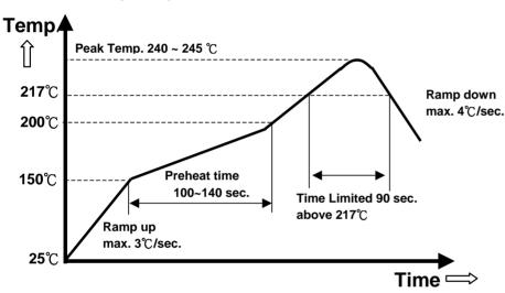
Note: The temperature refers to the pin of E36SC12009, measured on the +Vout pin joint.
