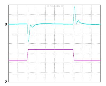
Figure 6: Output voltage response to step-change in load current (50%-75%-50% of lo, max; di/dt = 0.1A/μs; Vin is 24V). Load cap: 10μF tantalum capacitor and 1μF ceramic capacitor. Top Trace: Vout (0.2V/div, 200us/div), Bottom Trace:lout (2A/div). Scope measurement should be made using a BNC cable (length shorter than 20 inches). Position the load between 51 mm to 76 mm (2 inches to 3 inches) from the module
