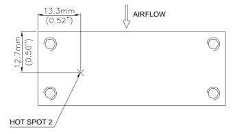
**Figure 22:** \* Hot spot 2 temperature measured point. The allowed maximum hot spot 2 temperature is defined at 105  $\mathcal C$
