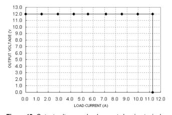
**Figure 13:** Output voltage vs. load current showing typical current limit curves and converter shutdown points (Vin=48V)
