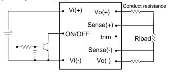
Figure 15: Effective circuit configuration for remote sense operation
