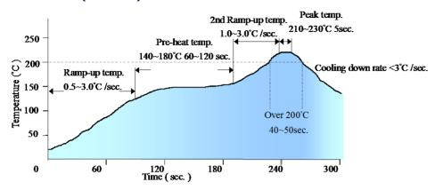
Note: The temperature refers to the pin of E36SC, measured on the +Vout pin joint.
