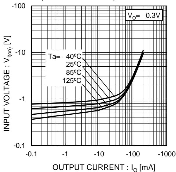
Fig.2 Output current vs. input voltage
