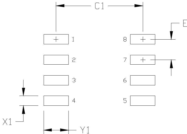
**Figure 19. PCB Land Pattern: 8-Pin Narrow Body SOIC**
