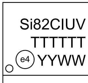
Figure 23. 8-Pin Narrow Body SOIC Top Marking
