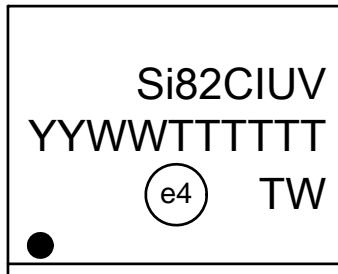
Figure 22. 16-Pin Wide Body SOIC Top Marking
