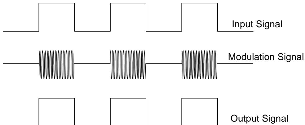
**Figure 7. Modulation Scheme**
