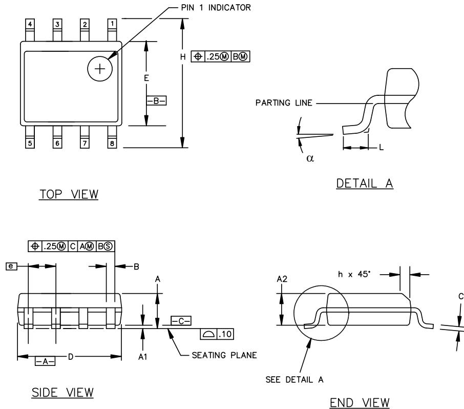
**Figure 18. 8-pin Small Outline Integrated Circuit (SOIC) Package**
