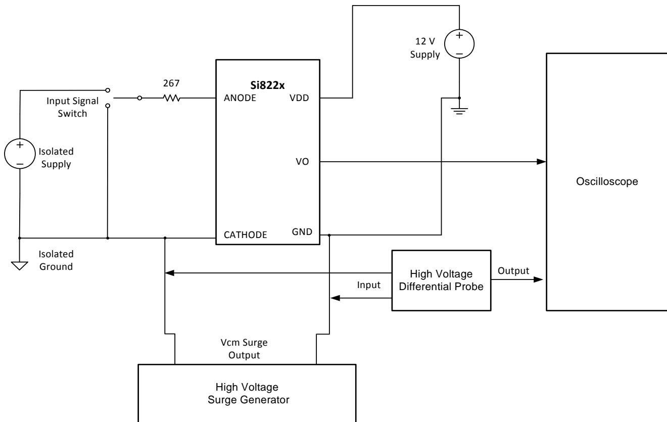
Figure 3. Common Mode Transient Immunity Test Circuit
