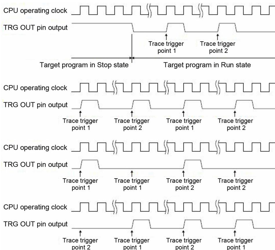
**Fig. 4 Examples of TRG OUT output timing**
