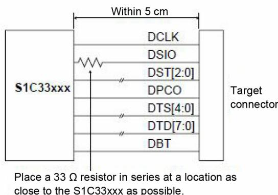
**Fig. 11 Wiring between S1C33xxx and target connector**
