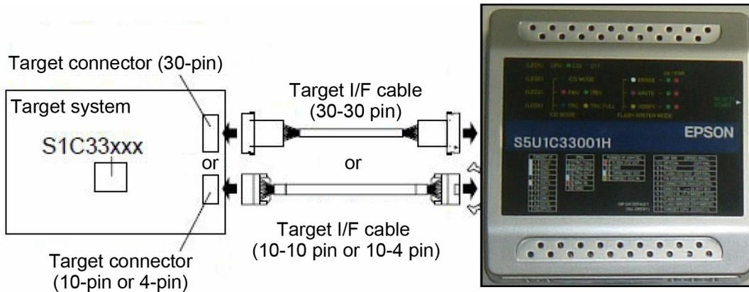
Fig. 8 Connecting the target system
