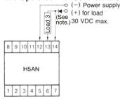
Note: Connect a diode when using a Power Supply of 12 V or less.
