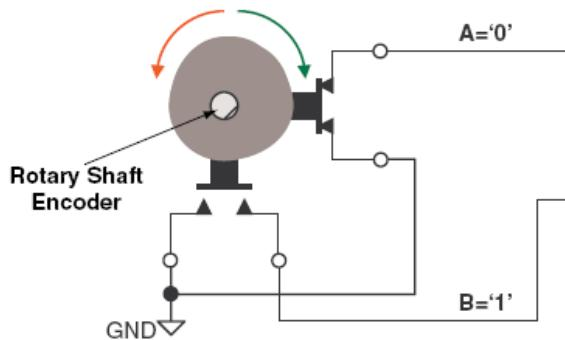
Figure 1. Rotary shaft encoder circuitry.
