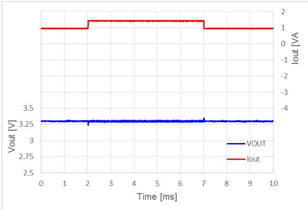
**RP602Z330x,  $V_{IN} = 3.6 \text{ V}$ , MODE = L**
