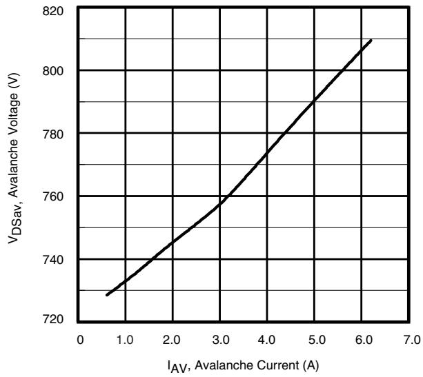
Fig. 12d - Typical Drain-to-Source Voltage vs. Avalanche Current
