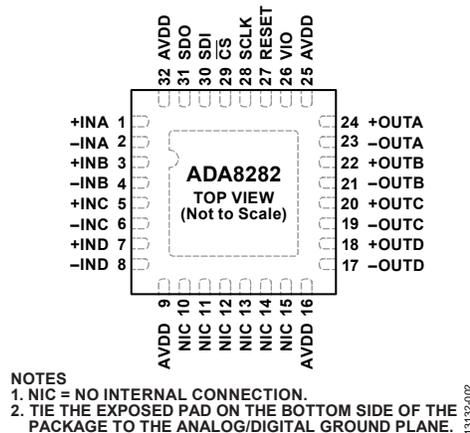
Figure 2. Pin Configuration
