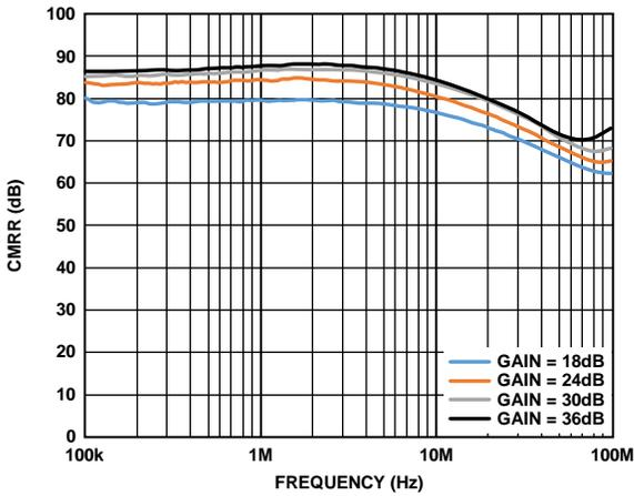
Figure 22. CMRR vs. Frequency at Various Gains
