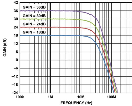
Figure 12. Frequency Response at All Gains (Bias Mode 0)
