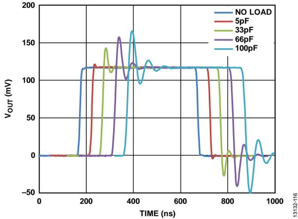
Figure 15. Pulse Response at Various Output Capacitive Loads
