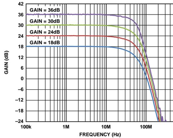
Figure 13. Frequency Response at All Gains (Bias Mode 2)
