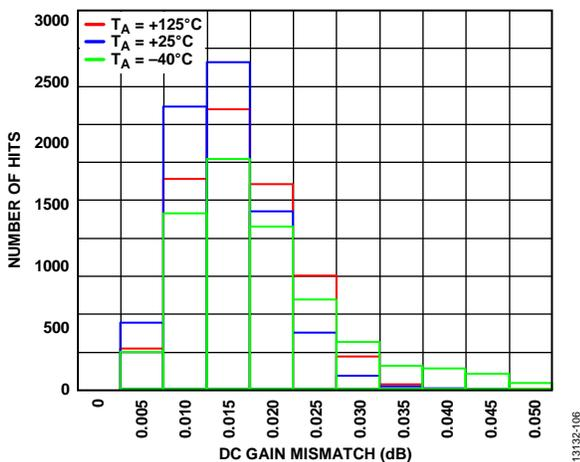
Figure 5. Distribution of Channel to Channel Gain Matching
