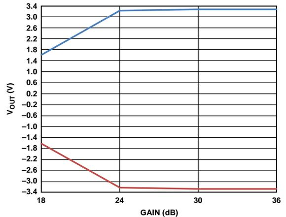
Figure 19. Maximum and Minimum Differential  $V_{OUT}$  vs. Gain
