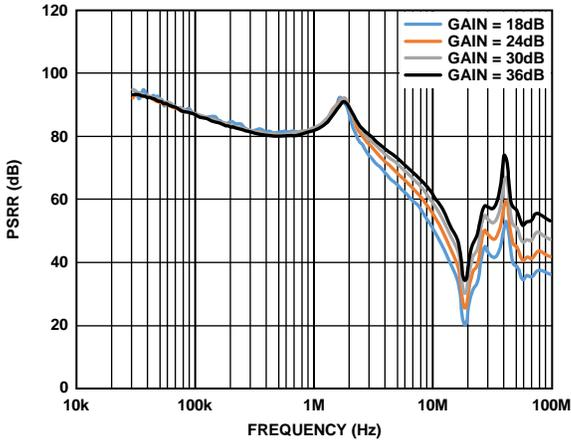
Figure 21. PSRR vs. Frequency at Various Gains
