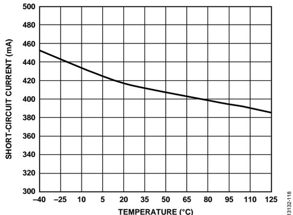
Figure 17. Short-Circuit Current vs. Temperature Per Channel
