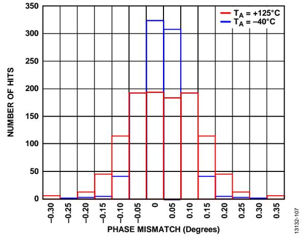
Figure 6. Distribution of Channel to Channel Phase Matching
