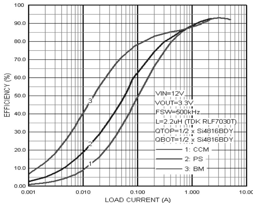
Figure 3. Efficiency vs load current For Vout1
