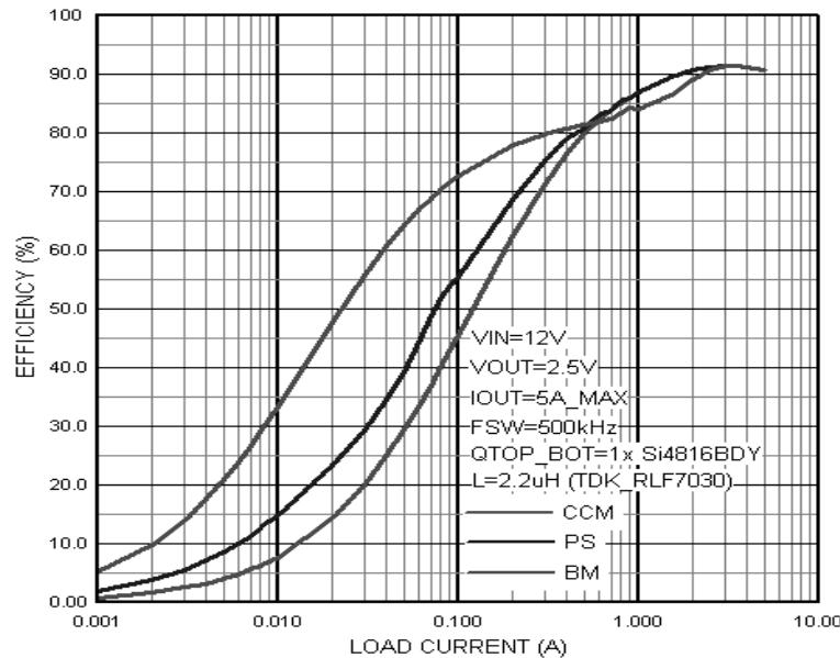
Figure 4. Efficiency vs load current For Vout2
