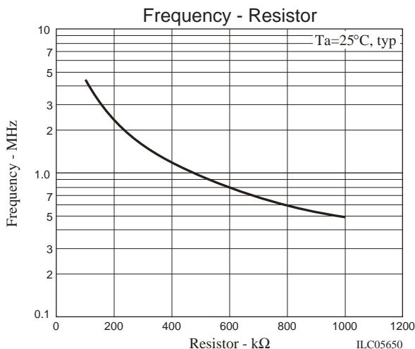
Figure 8 Characteristics of Resistor v.s. Frequency of OSC1
