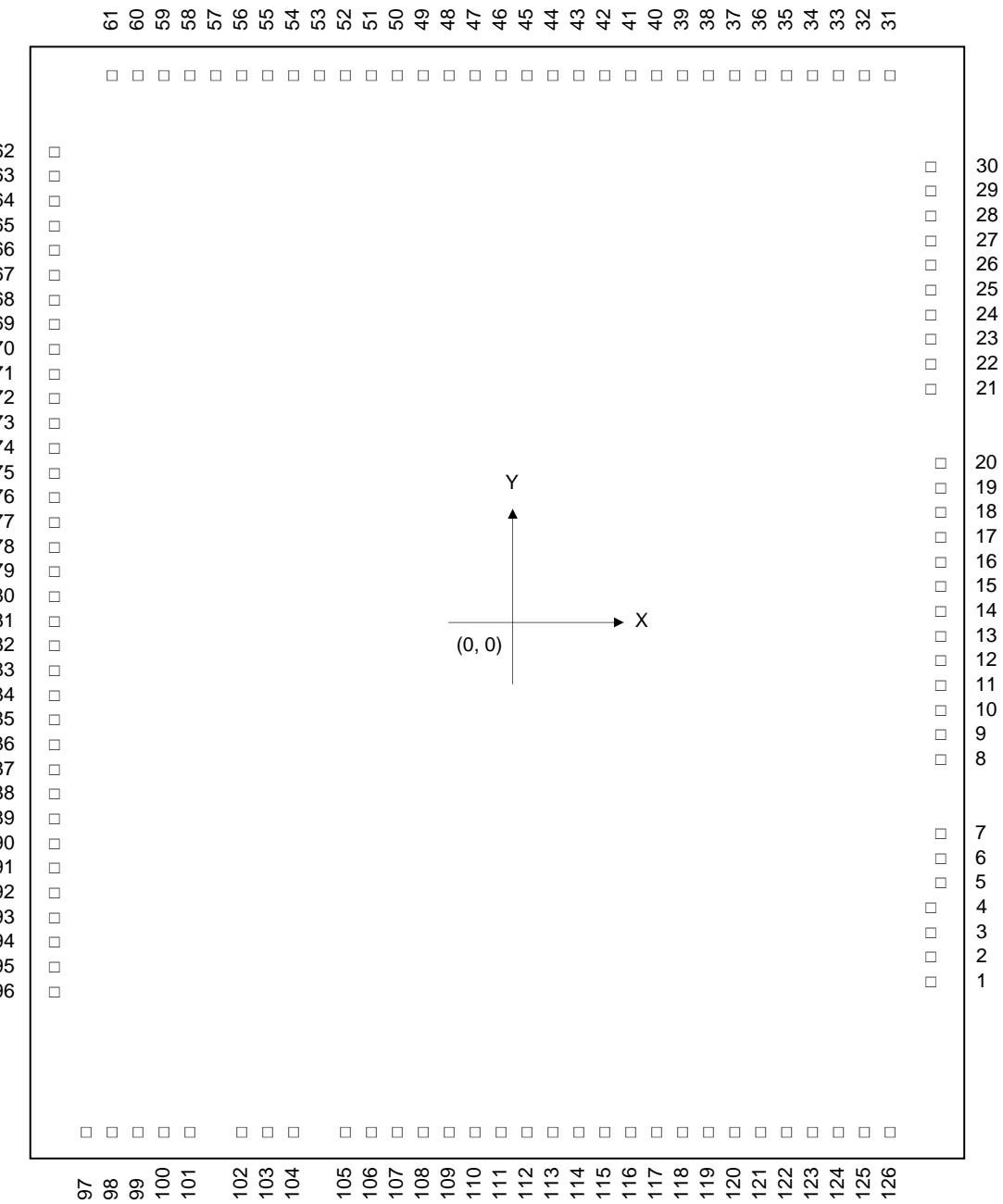
Note: Pin numbers assigned to a package differ from pad numbers assigned to a chip.
