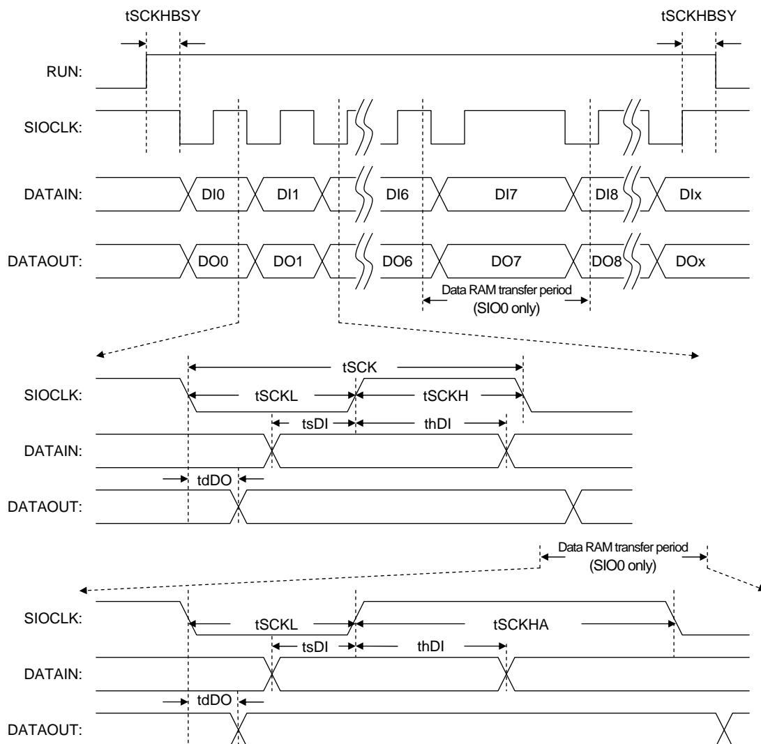
\*: Remarks:  $D_{Ix}$  and  $D_{Ox}$  are the final communication bits.  $X = 0$  to 32768
