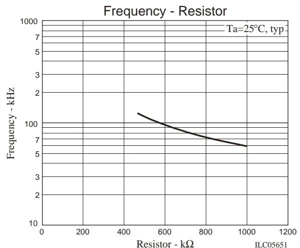
Figure 9 Characteristics of Resistor v.s. Frequency of OSC0
