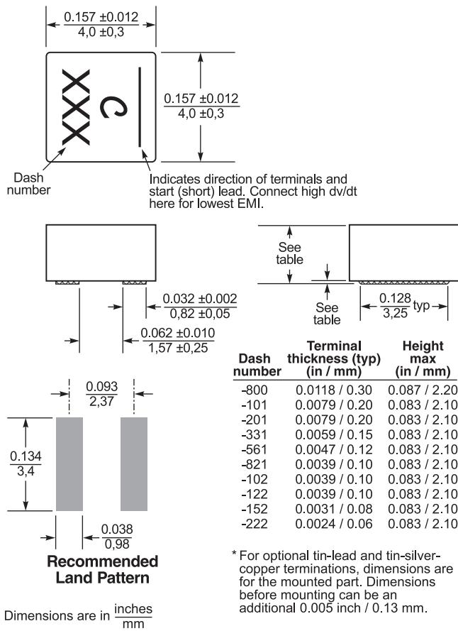
\* For optional tin-lead and tin-silver-copper terminations, dimensions are for the mounted part. Dimensions before mounting can be an additional 0.005 inch / 0.13 mm.
