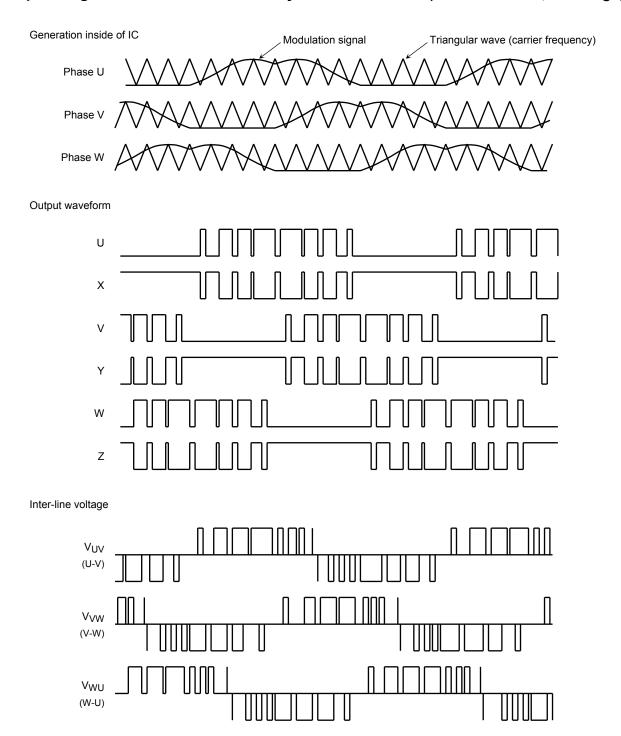
When the motor is driven by a sine wave, the motor is accelerated or decelerated according to the On duty of  $T_{ONU}$  when the amplitude of the modulation symbol changes by voltage  $V_e$  (see the diagram of output On duty on page 11):
