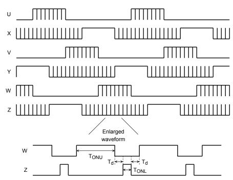
To stabilize the bootstrap voltage, the lower outputs (X, Y, and Z) are always turned on at the carrier cycle even during off time. At that time, the upper outputs (U, V, and W) are assigned dead time and turned off at the timing when the lower outputs are turned on.  $(T_d \text{ varies with input } V_e)$
