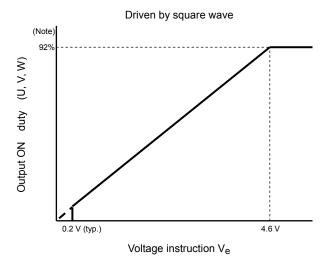
Note: Output ON time is decreased by the dead time (carrier frequency  $\times$  92% - T<sub>d</sub>  $\times$  2).
