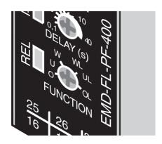
If an error is present when the monitoring module is activated, output relay "R" remains dropped out and the LED for the corresponding threshold value lights up.
