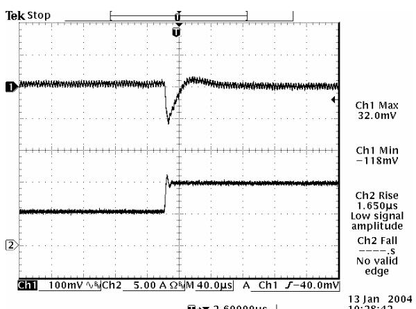
50% to 100% load step at 1.5 V output
