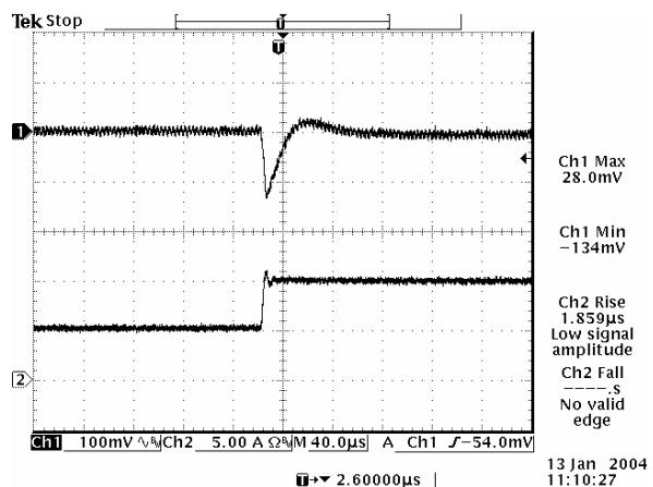
50% to 100% load step at 1.2 V output
