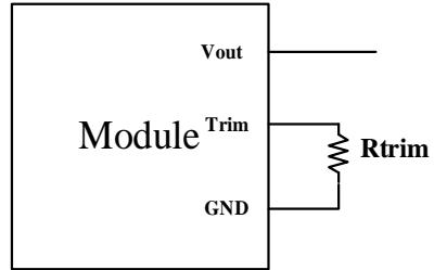
Equation for calculating the trim voltage (in V) given the desired adjusted voltage ( $V_{adj}$ ) is shown below. The Trim Up voltage should be connected between the Trim pin and Ground.
