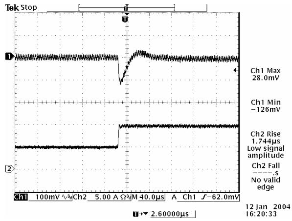
50% to 100% load step at 3.3 V output
