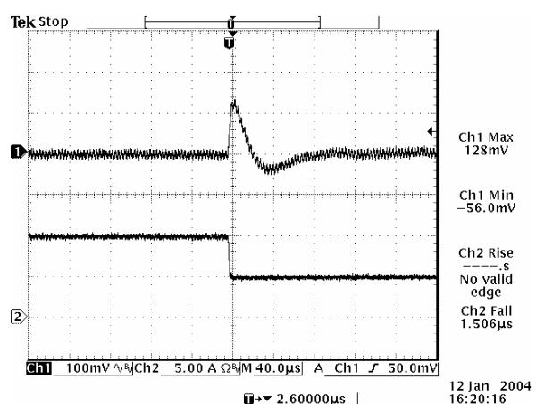
100% to 50% load step at 3.3 V output
