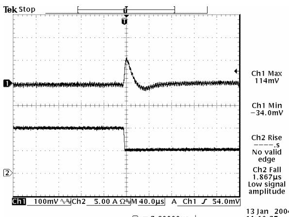
100% to 50% load step at 1.2 V output
