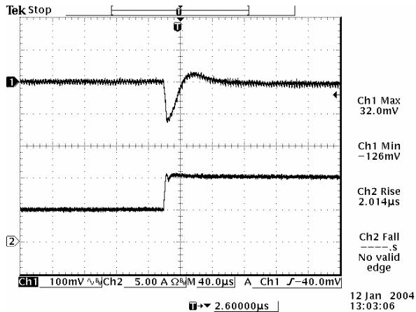
50% to 100% load step at 0.75 V output
