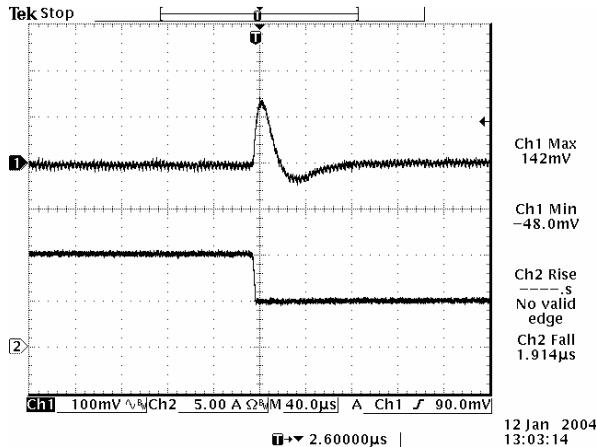
100% to 50% load step at 0.75 V output
