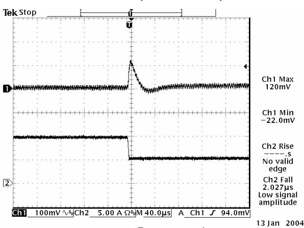
100% to 50% load step at 1.5 V output
