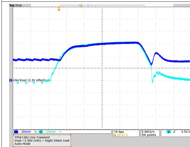
Figure 43. TPS61281 Forced Pass-Through to Boost Mode Transition
