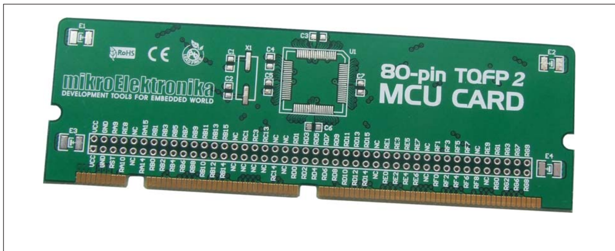
Figure 7: Empty 80-pin MCU card (TQFP2)
