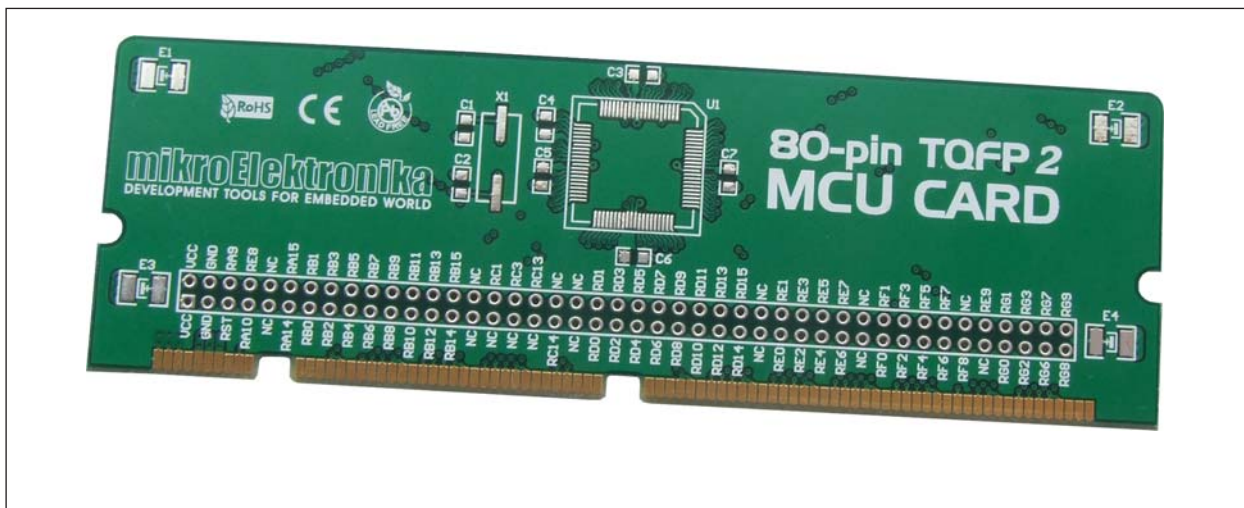
Figure 7: Empty 80-pin MCU card (TQFP2)
