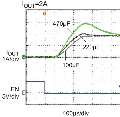
**1Ω Load Connected to Enabled Device**
