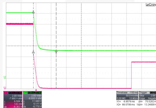
Figure 48. C2[V<sub>BLD</sub>], C4[V<sub>o</sub>] 90 V<sub>AC</sub> / 60 Hz & I<sub>o</sub>=0 A, 12 V to 5 V
