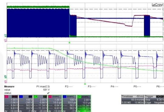
Figure 34. C2[FB], C3[V<sub>DS</sub>], C4[VO] 264 V<sub>AC</sub>/50 Hz, 12 V, Full Load Output Short
