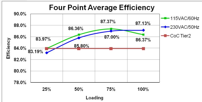
**Figure 70.** Efficiency at 9 V/1.5 A (Fixed Output Current Setting)
