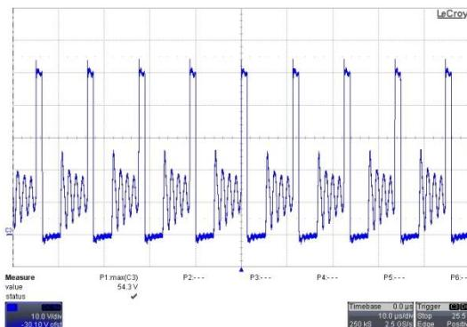
Figure 33. C3[V<sub>DS</sub>], 264 V<sub>AC</sub>/50 Hz, 12 V, Full Load
