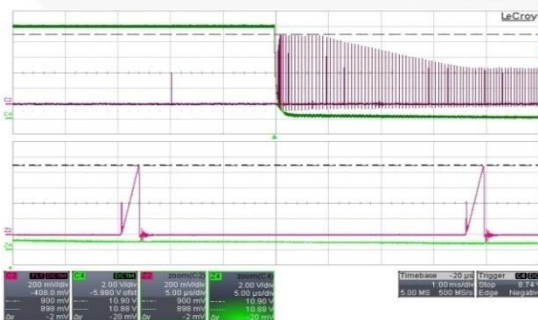
Figure 29. C2[V Cs ], C4[V O ], 264 V AC /50 Hz, I O =0 A, V O =12 V
