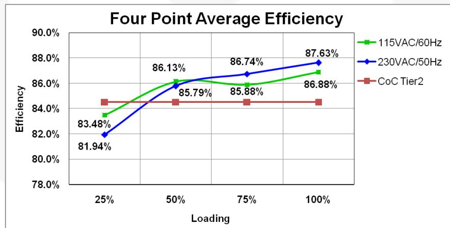
Figure 43. 12 V Efficiency Curve (4 Point Average: 100%, 75%, 50%, 25%)
