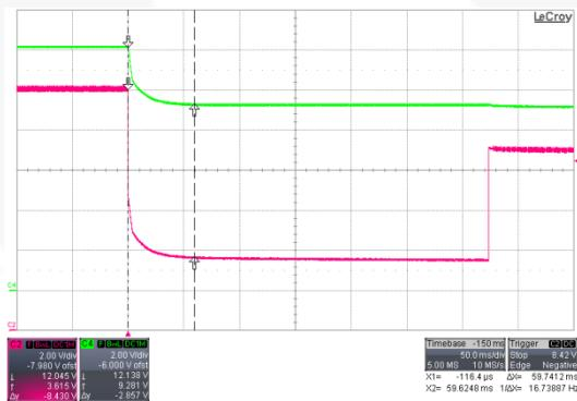
Figure 49. 90 V<sub>AC</sub> / 60 Hz & I<sub>o</sub>=0 A, 12 V to 9 V
