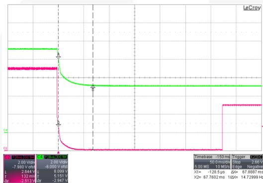
Figure 47. C2[V<sub>BLD</sub>], C4[V<sub>o</sub>] 90 V<sub>AC</sub> / 60 Hz & I<sub>o</sub>=0 A, 9 V to 5 V
