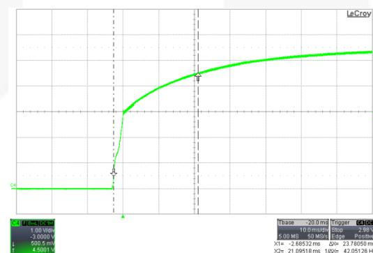
Figure 16. C4[Vo] 264 V<sub>AC</sub>/50 Hz, Full Load
