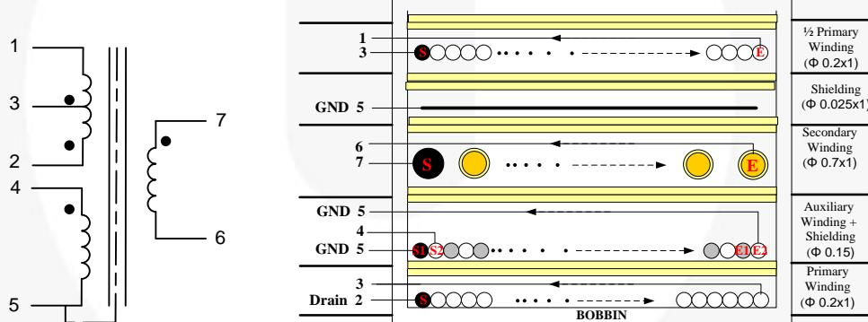
Figure 7. Transformer Specifications & Construction
