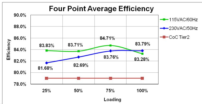
Figure 41. 5 V Efficiency Curve (4 Point Average: 100%, 75%, 50%, 25%)
