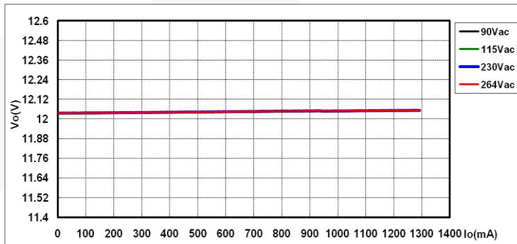
Figure 40. 12 V CV Deviation Curve
