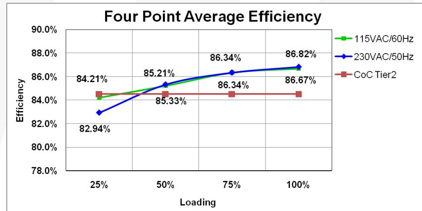
Figure 42. 9 V Efficiency Curve (4 Point Average: 100%, 75%, 50%, 25%)
