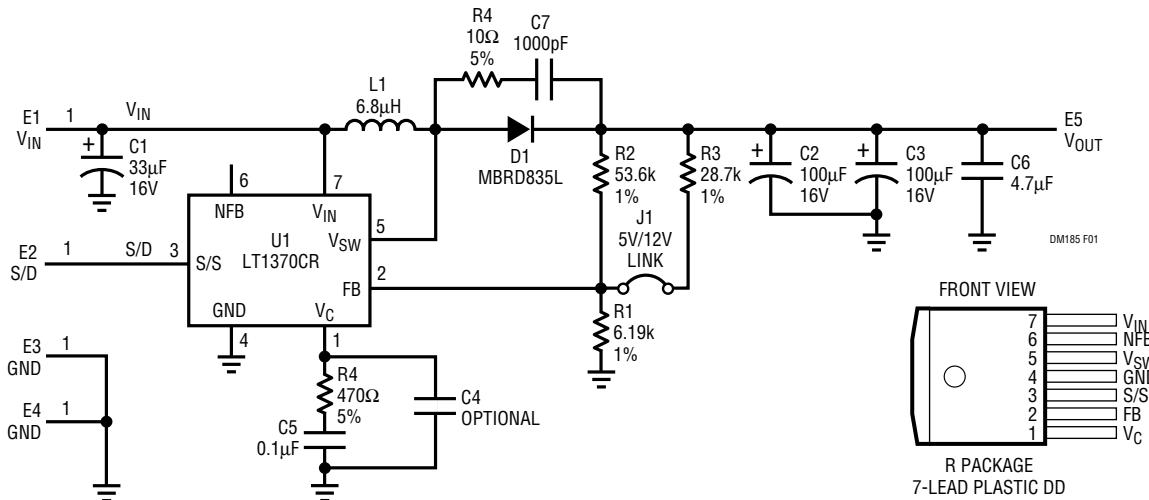
Figure 1. 5V/12V Output Boost Converter
