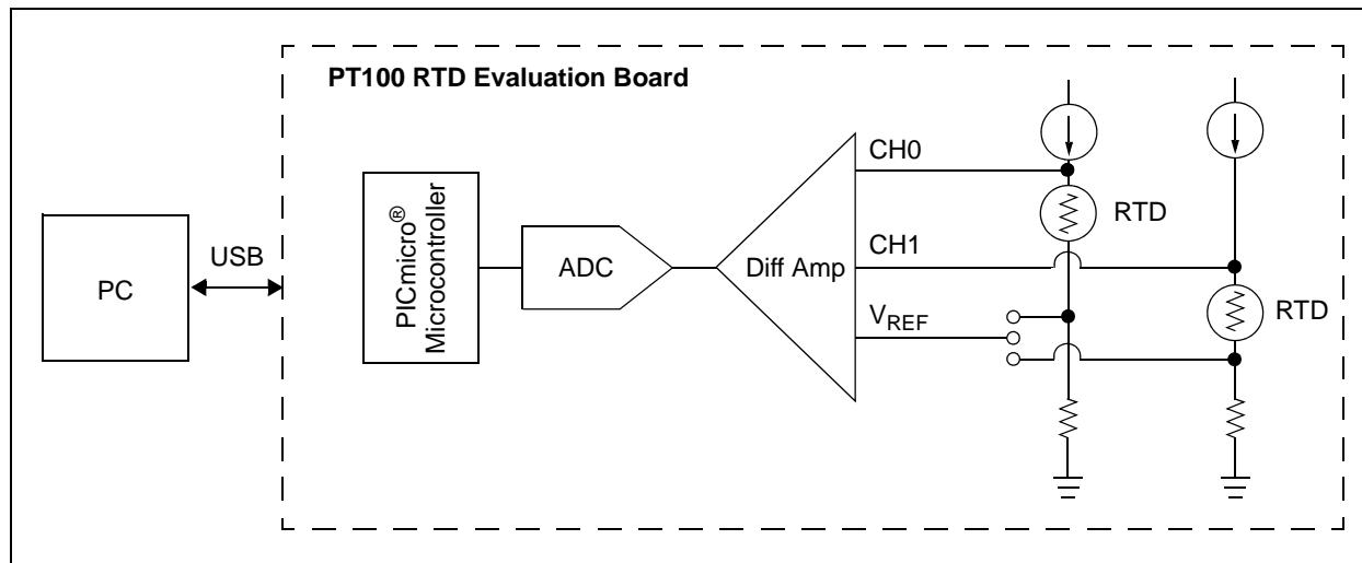
**FIGURE 2-1:** PT100 RTD Evaluation Board Simplified Block Diagram.
