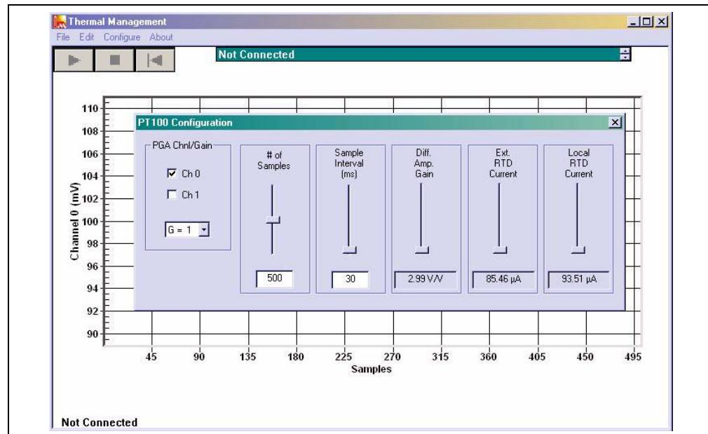
**FIGURE 2-3:** PC Software GUI.
