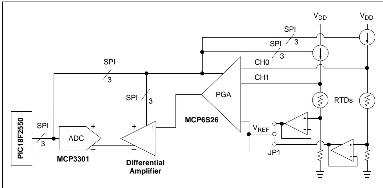
**FIGURE 2-2:** Simplified PT100 RTD Evaluation Board Schematic.
