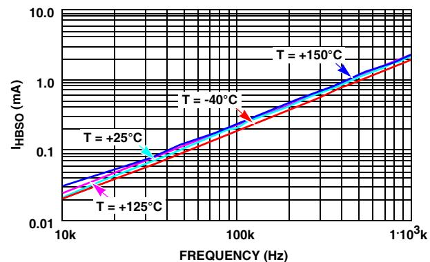
FIGURE 10.  $I_{HBS}$  OPERATING CURRENT vs FREQUENCY
