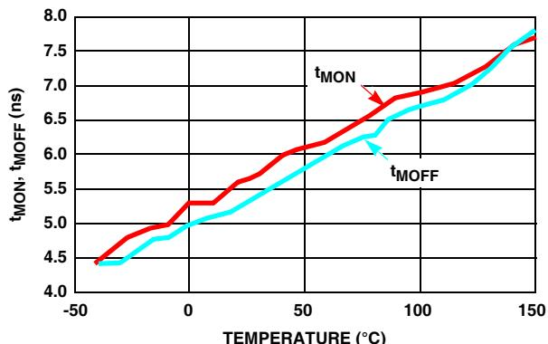
FIGURE 17. ISL2110 DELAY MATCHING vs TEMPERATURE
