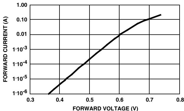
FIGURE 23. BOOTSTRAP DIODE I-V CHARACTERISTICS
