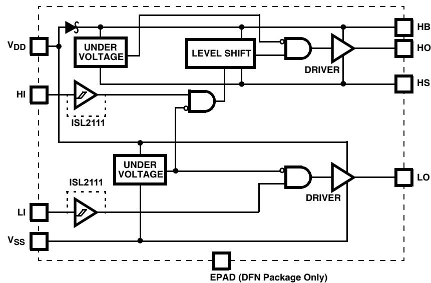
\*EPAD = Exposed Pad. The EPAD is electrically isolated from all other pins. For best thermal performance, connect the EPAD to the PCB power ground plane.
