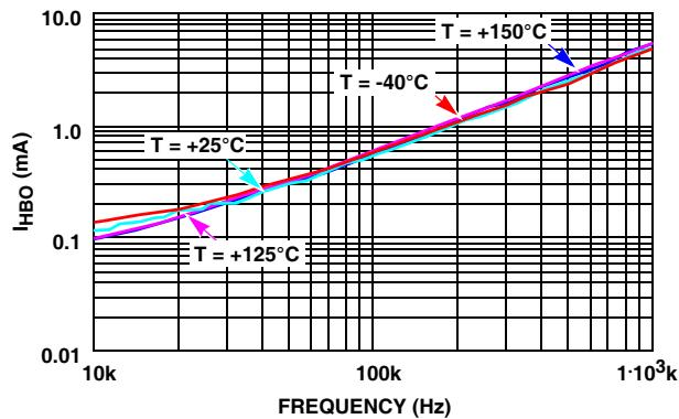
FIGURE 9.  $I_{HB}$  OPERATING CURRENT vs FREQUENCY
