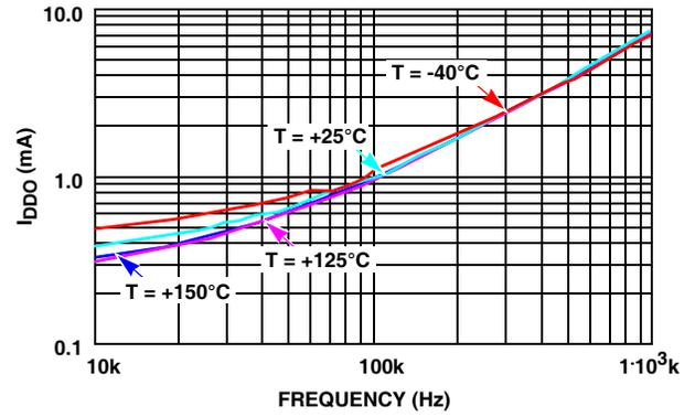
FIGURE 8. ISL2111  $I_{DD}$  OPERATING CURRENT vs FREQUENCY
