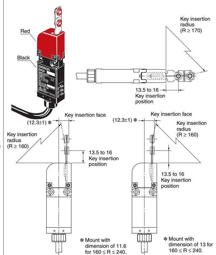
**Note:** Unless otherwise specified, a tolerance of  $\pm 0.4$  mm applies to all dimensions. Dimensions in parentheses are reference values.
