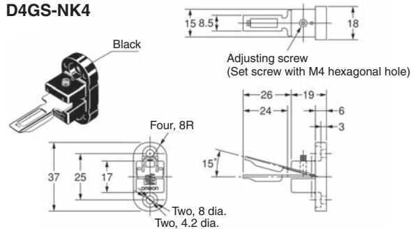
**Note:** Unless otherwise specified, a tolerance of  $\pm 0.4$  mm applies to all dimensions. Dimensions in parentheses are reference values.
