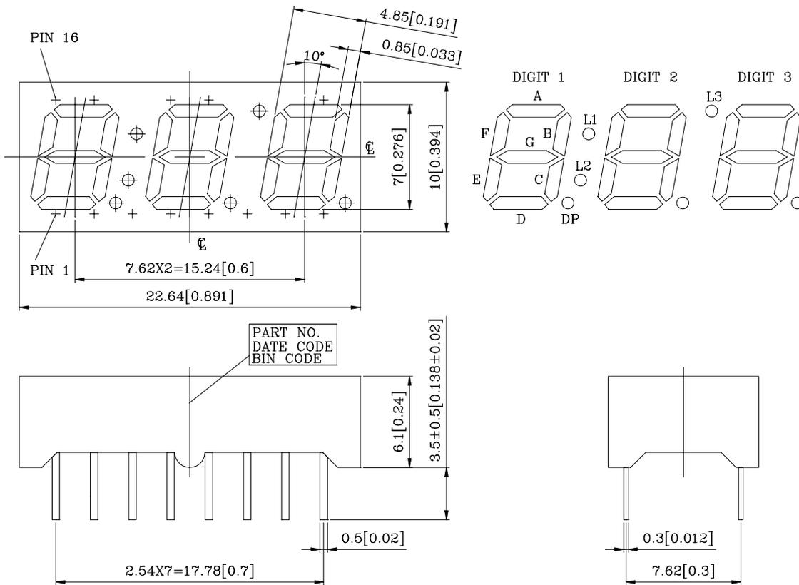
NOTES: All dimensions are in millimeters. Tolerances are ± 0.25 mm (0.01") unless otherwise noted.
