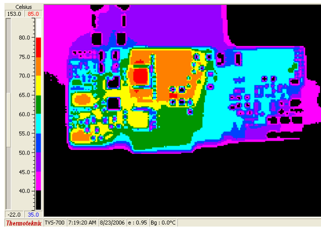
Figure 11. Temp Data (72Vin, 20A, 25°C, 200LFM airflow – back)
