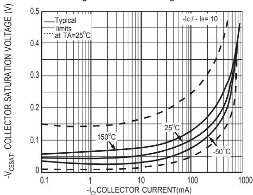
Figure 3 Collector Sat Voltage vs Collector Current
