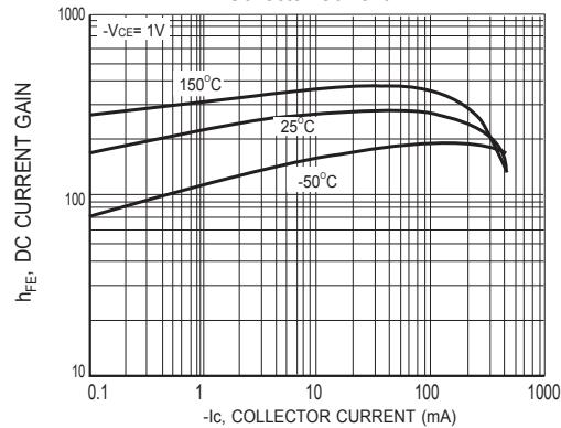
Figure 4 DC Current Gain vs Collector Current
