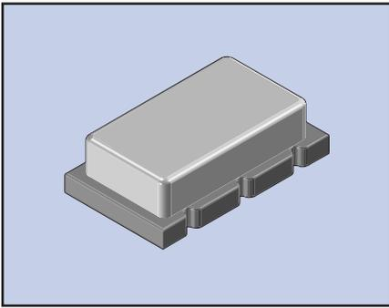
The ECS-SR-B Series SMD ceramic resonator includes built-in capacitors for simplification of oscillator circuits and reduces component count. The SMD ceramic resonator is an excellent low cost frequency control solution when absolute frequency accuracy is not important.
