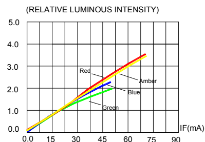
FIG.2 RELATIVE LUMINOUS INTENSITY VS. FORWARD CURRENT
