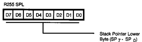
Figure 37. Stack Pointer (FF<sub>H</sub>: Read/Write)
