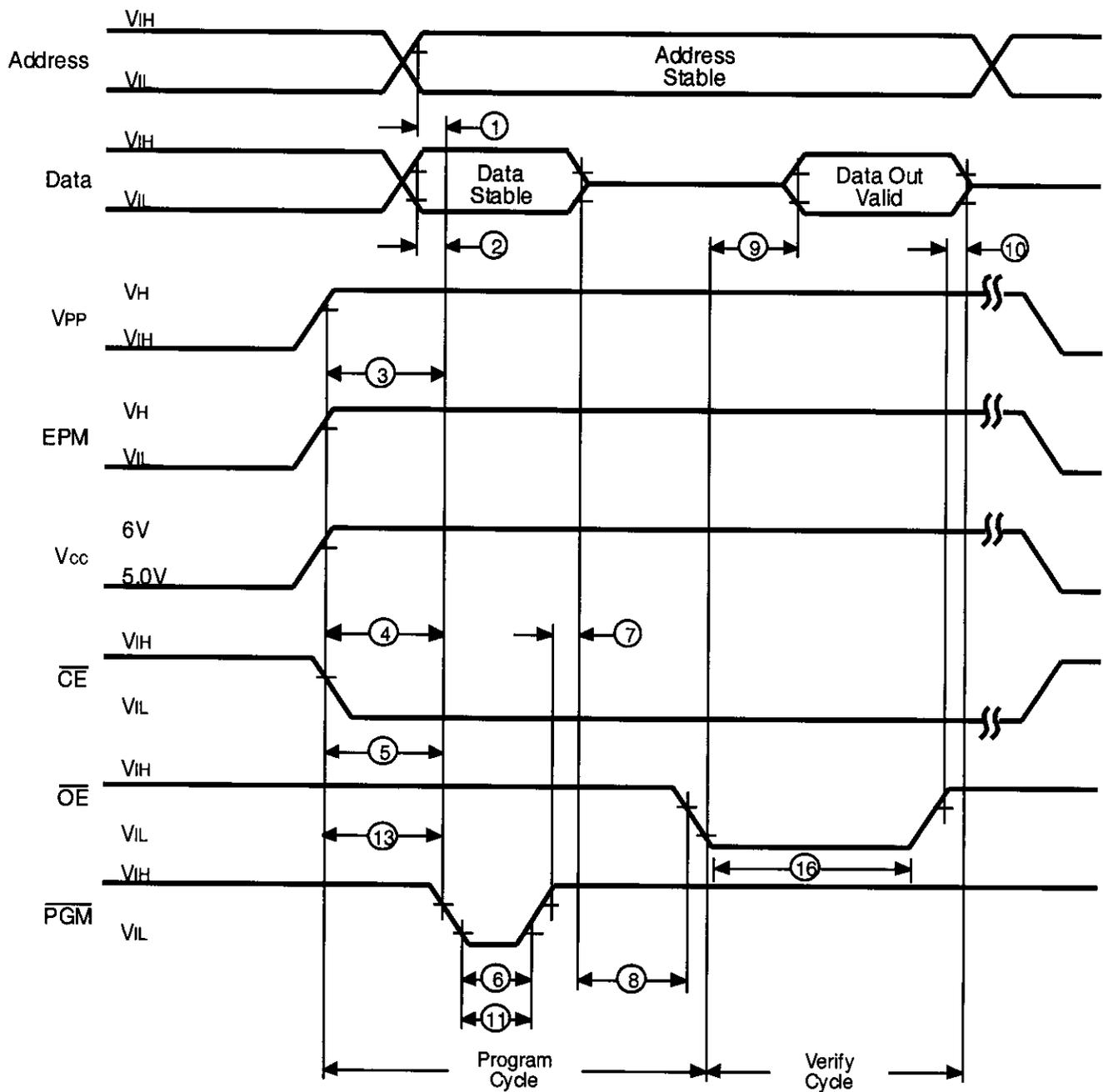
Figure 20. Z86E04/E08 Programming Waveform
