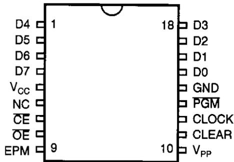
Figure 3. 18-Pin EPROM Mode Configuration
