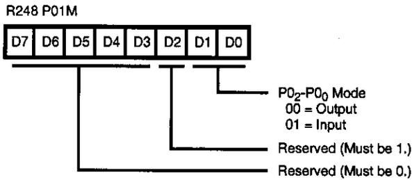
Figure 31. Port 0 and 1 Mode Register (F8<sub>H</sub>: Write Only)
