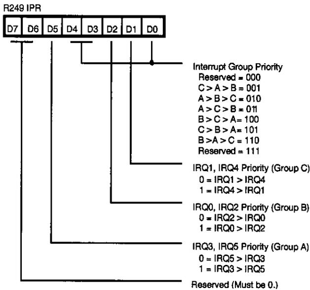
Figure 32. Interrupt Priority Register (F9<sub>H</sub>: Write Only)
