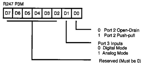
Figure 30. Port 3 Mode Register (F7<sub>H</sub>: Write Only)
