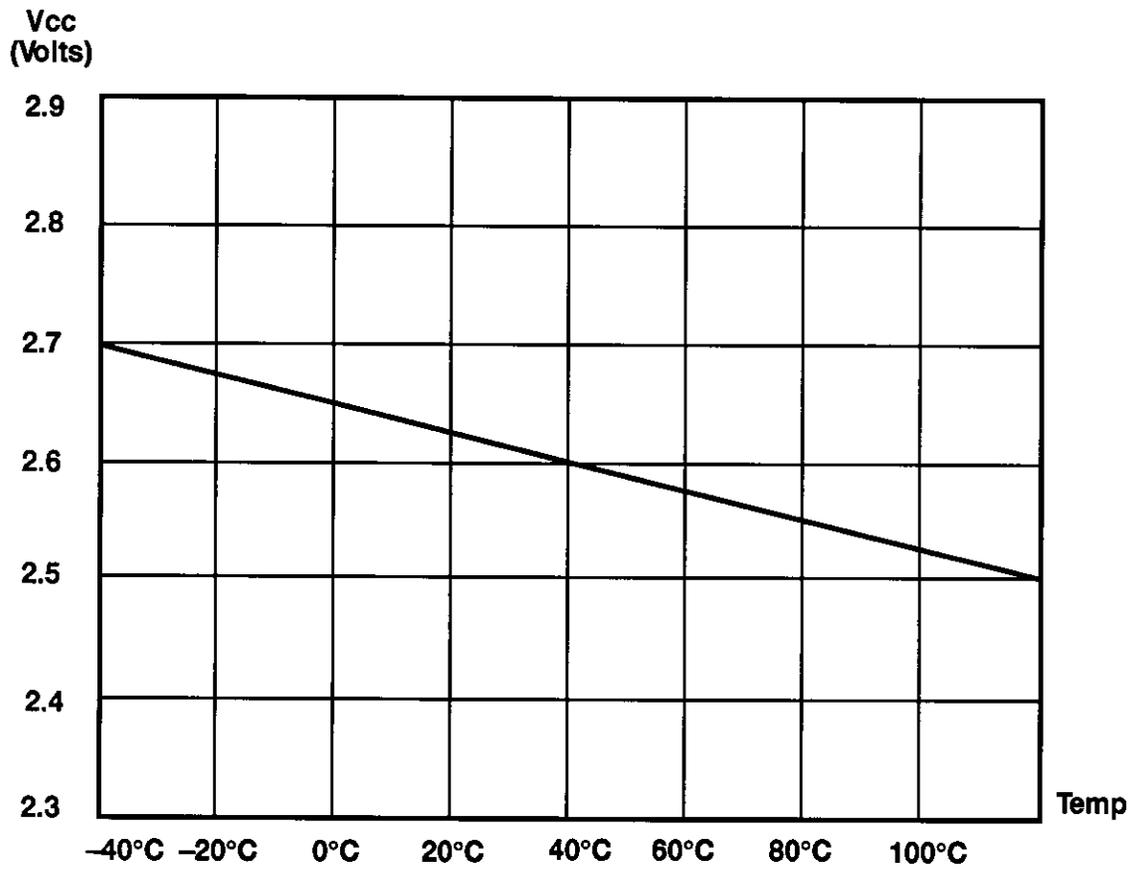
Figure 17. Typical Auto Reset Voltage ( $V_{LV}$ ) vs. Temperature
