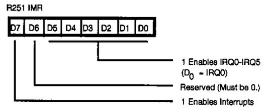
Figure 34. Interrupt Mask Register (FB<sub>H</sub>: Read/Write)
