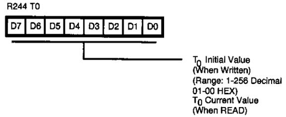
Figure 27. Counter/Timer 0 Register (F4<sub>H</sub>: Read/Write)
