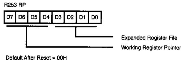
Figure 36. Register Pointer (FD<sub>H</sub>: Read/Write)
