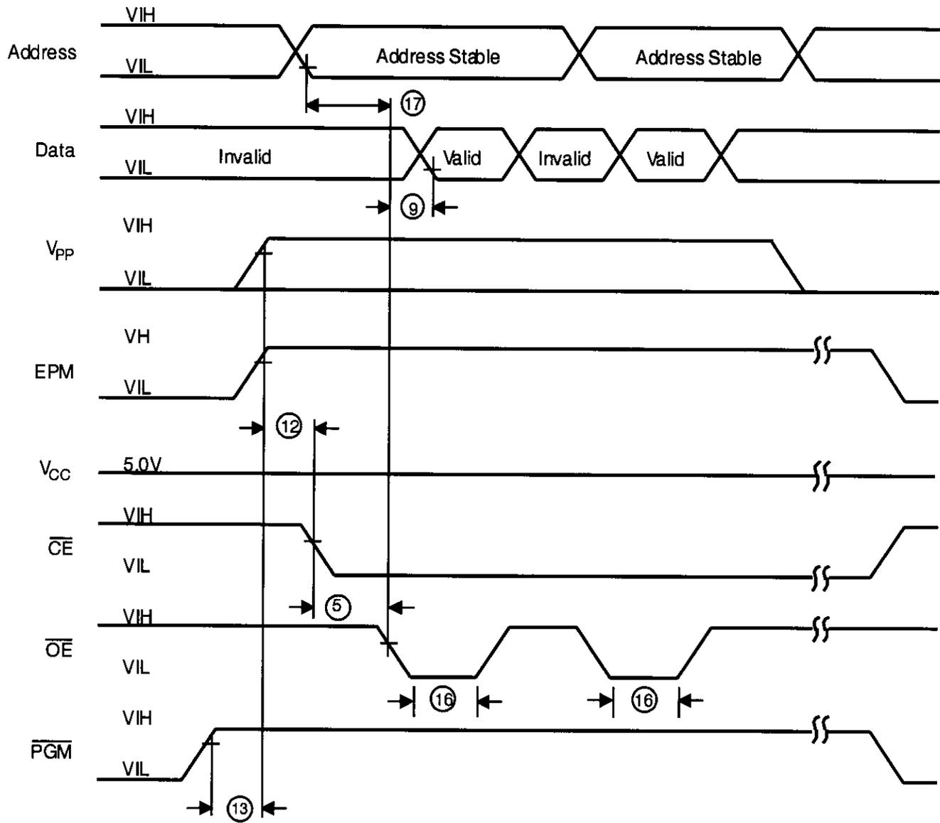
Figure 19. Z86E04/E08 Programming Waveform
