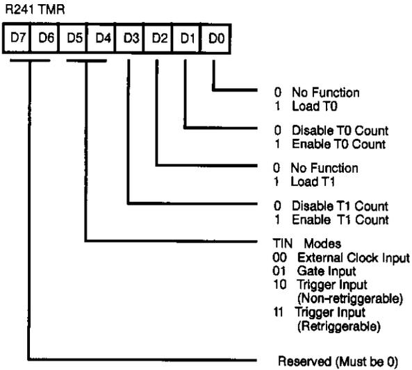
Figure 24. Timer Mode Register (F1<sub>H</sub>: Read/Write)
