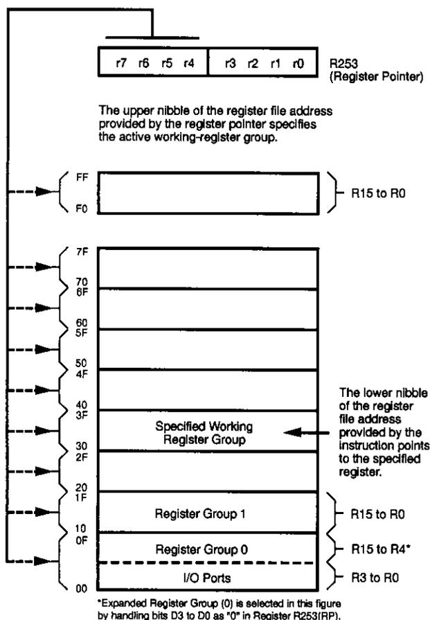
Figure 13. Register Pointer
