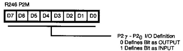
Figure 29. Port 2 Mode Register (F6<sub>H</sub>: Write Only)
