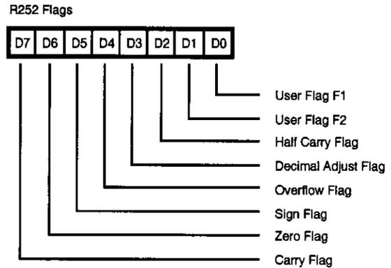
Figure 35. Flag Register (FC<sub>H</sub>: Read/Write)
