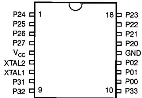
Figure 4. 18-Pin DIP/SOIC Mode Configuration
