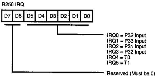
Figure 33. Interrupt Request Register (FA<sub>H</sub>: Read/Write)
