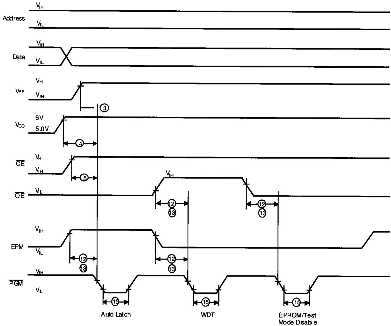
**Figure 22. Z86E04/E08 Programming Options Waveform
