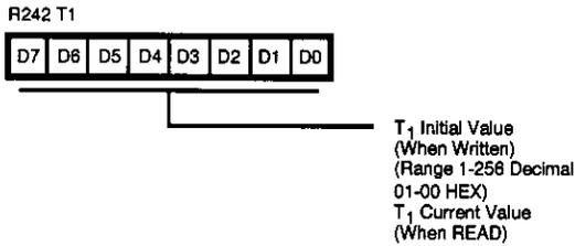
Figure 25. Counter Timer 1 Register (F2<sub>H</sub>: Read/Write)
