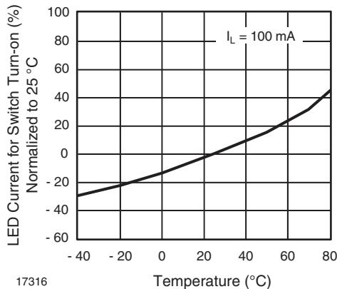
Fig. 17 - LED Current for Switch Turn-on vs. Temperature
