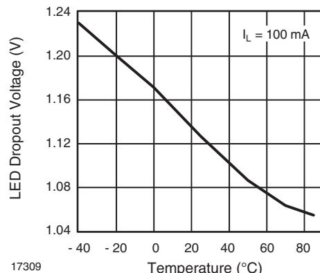
Fig. 10 - LED Dropout Voltage vs. Temperature
