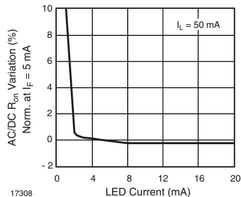
Fig. 9 - Variation in On-resistance vs. LED Current
