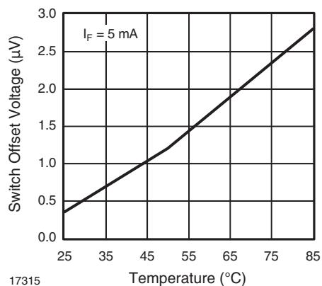
Fig. 16 - Switch Offset Voltage vs. Temperature
