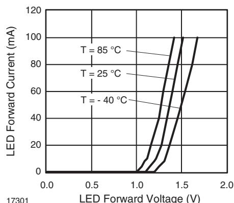
Fig. 2 - LED Forward Current vs. LED Forward Voltage
