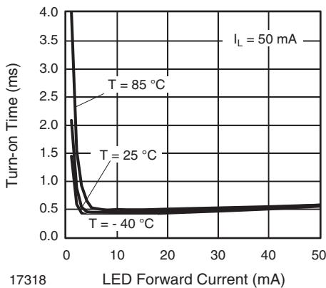
Fig. 19 - Turn-on Time vs. LED Current
