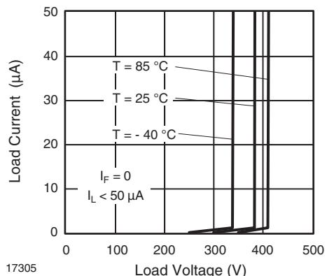
Fig. 6 - Switch Breakdown Voltage vs. Load Current
