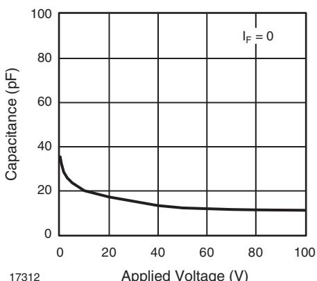
Fig. 13 - Switch Capacitance vs. Applied Voltage
