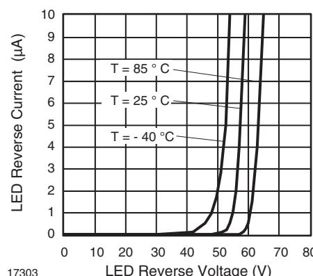
Fig. 4 - LED Reverse Current vs. LED Reverse Voltage
