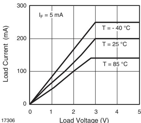
Fig. 7 - Load Current vs. Load Voltage
