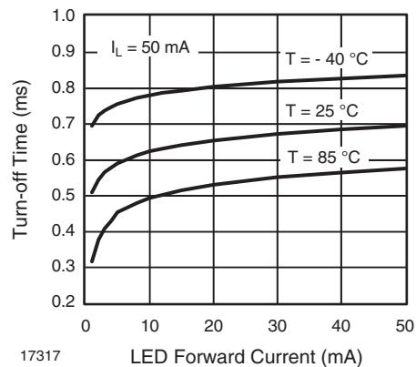
Fig. 18 - Turn-off Time vs. LED Current
