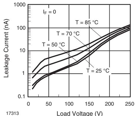
Fig. 14 - Leakage Current vs. Applied Voltage
