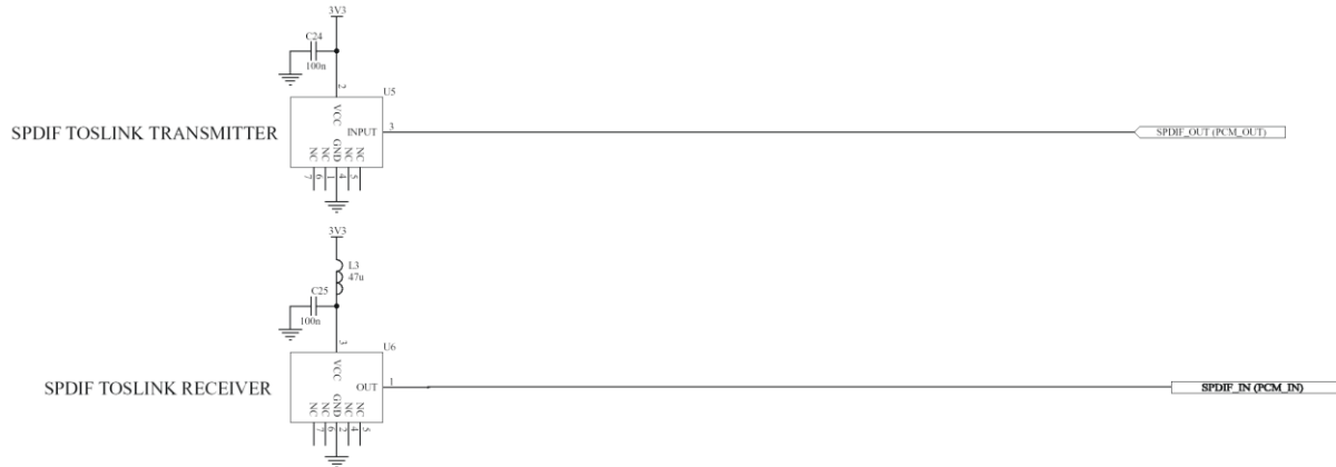
Figure 16: Example circuit for SPDIF interface (Optical)
