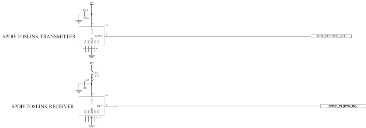
Figure 16: Example circuit for SPDIF interface (Optical)
