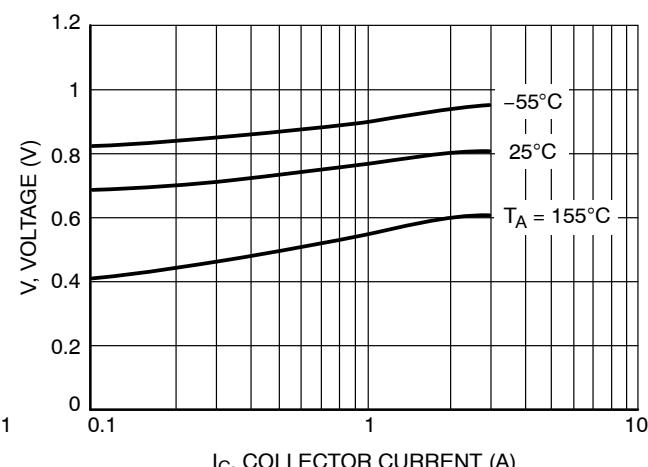
**Figure 6.  $V_{BE(on)}$  Voltage**
