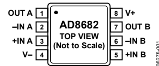
Figure 1. 8-Lead SOIC_N and 8-Lead MSOP
