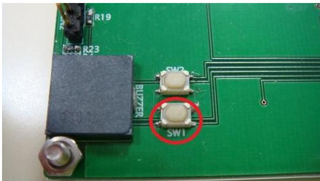
Figure 5: Reset Switch of LC717A10AR and LC898301XA
