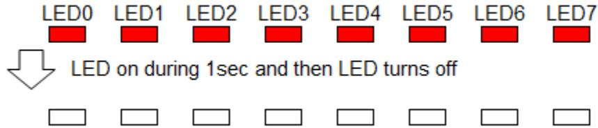
LED blinks three times when USB is connected if the USB driver is available. (USB driver is optional. It is necessary when updating the firmware.)
