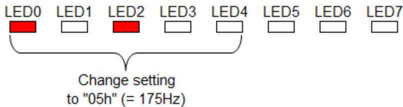
If current resonance frequency is 175Hz, then resonance frequency will change to 205Hz.
