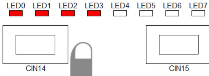
When close to CIN15 LEDs on right side turn ON.
