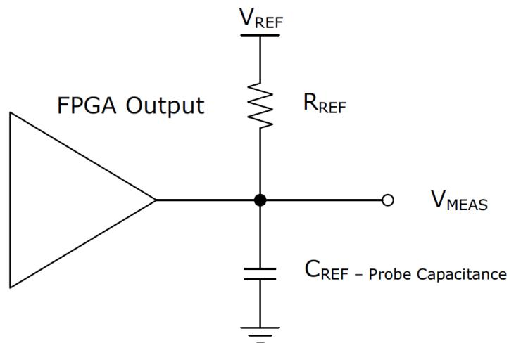
**Figure 2 • Output Delay Measurement—Differential Test Setup**
