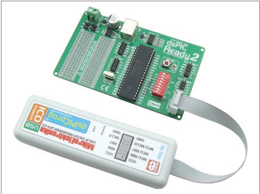
Figure 2: Programming the on-board microcontroller
