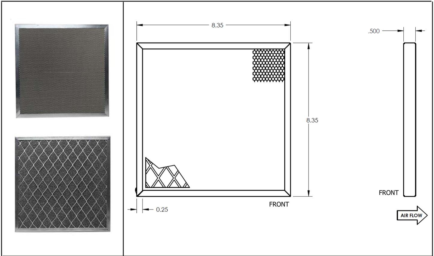
Orion Fans Pyrocide filters meet stringent flame safety standards for fire containment in electronics enclosures by preventing flames from propagating through the vent panels. The pyrocide coating has an ASTM E-84 Class A rating with low flame spread and low smoke index values. A thin coating in the honeycomb cells reacts on exposure to flame and expands rapidly, to prevent flames from propagating through the vent panels.
