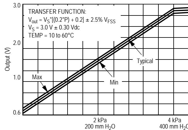
**Figure 4. Output vs. Pressure Differential at  $\pm 2.5\% V_{FSS}$**
