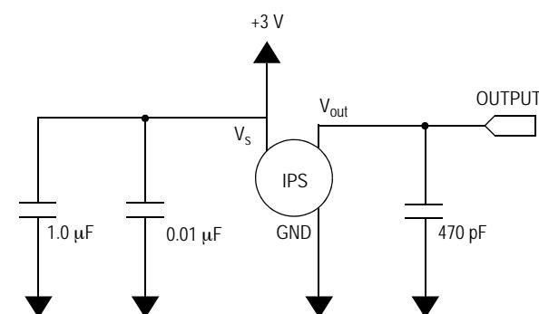
**Figure 3. Recommended Power Supply Decoupling and Output Filtering.**
