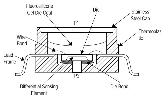
**Figure 2. Cross Sectional Diagram SSOP (not to scale)**
