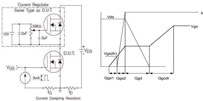
Fig 14a&b. Basic Gate Charge Test Circuit
