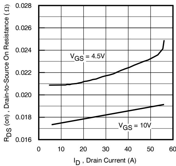
Fig 12. Typical On-Resistance Vs.
