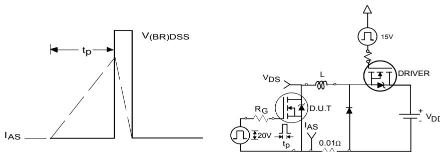
Fig 15a&b. Unclamped Inductive Test circuit
