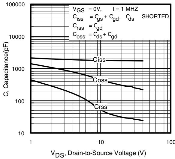
**Fig 5.** Typical Capacitance vs.
