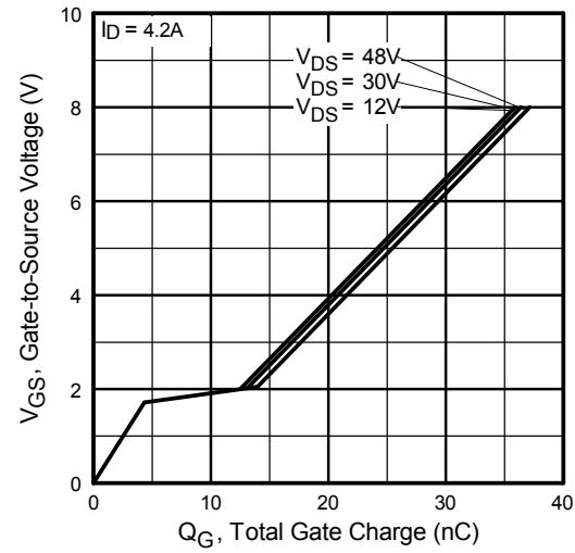
**Fig 6.** Typical Gate Charge vs.
