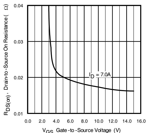
Fig 13. Typical On-Resistance Vs.
