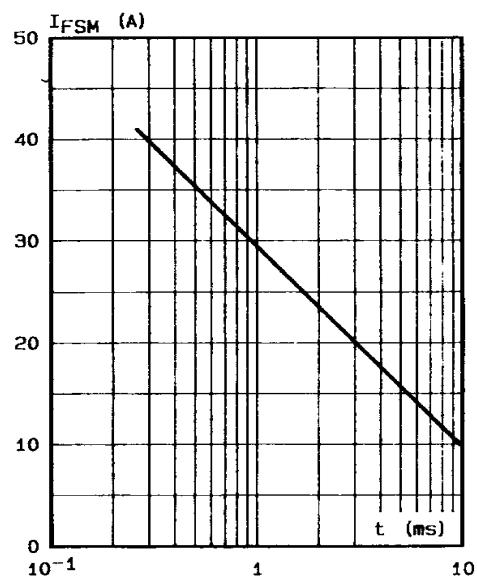
**Figure 7. Surge non repetitive forward current versus number of cycles.**
