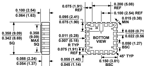
CONTROLLING DIMENSIONS ARE IN INCHES; MILLIMETER DIMENSIONS
