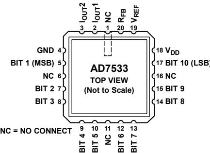
Figure 5. 20-Terminal LCC Pin Configuration
