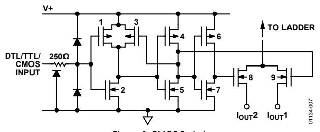
Figure 8. CMOS Switch
