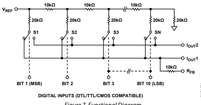
Figure 7. Functional Diagram
