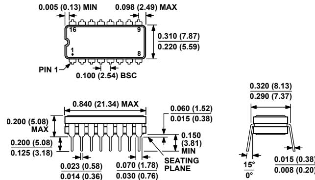
CONTROLLING DIMENSIONS ARE IN INCHES; MILLIMETER DIMENSIONS
