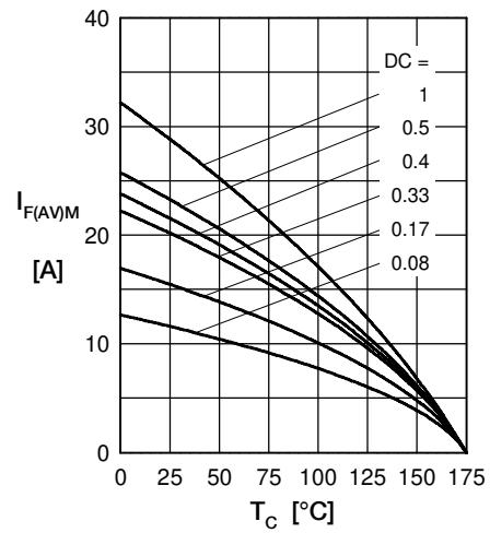
Fig. 5 Max. forward current vs.
