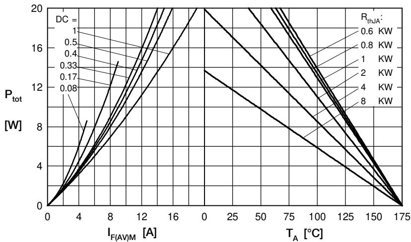
Fig. 4 Power dissipation vs. forward current
