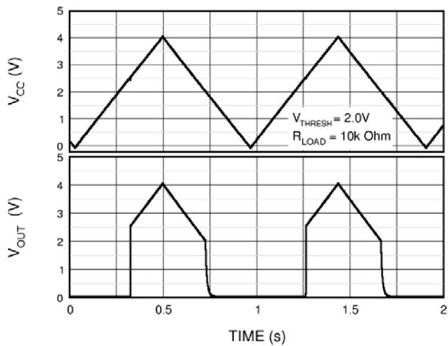
**Figure 2.2 On Mode Switching Behavior**
