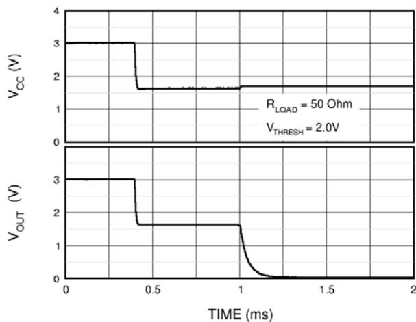
**Figure 2.6 Over-Current Retry Performance**
