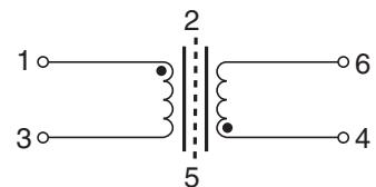
Note: For T6074 connection of shield, ground pin 2 or 5, not both pins
