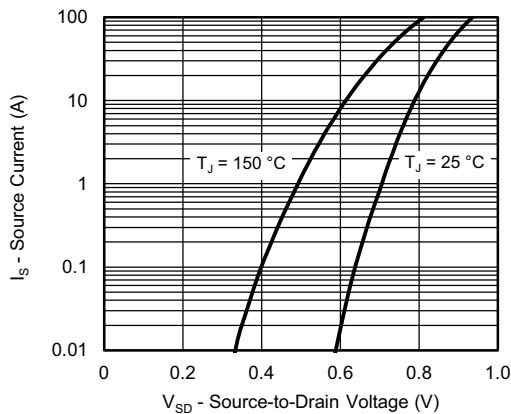
**Source-Diode Forward Voltage**
