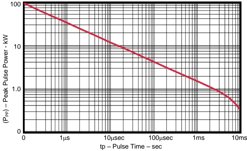
FIGURE 1 – Peak Pulse Power vs. Pulse Time
